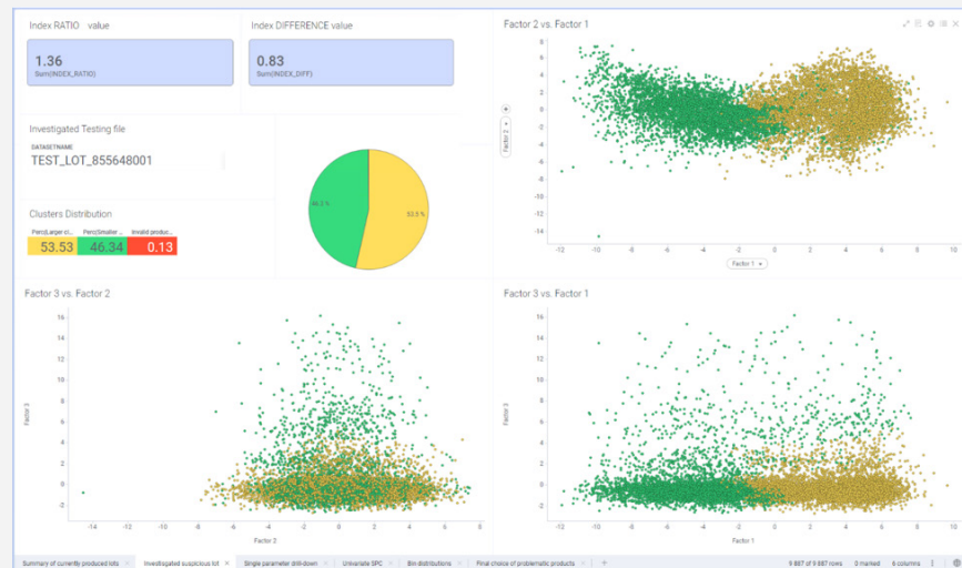
Figure 4. Interactive visual investigation of the suspicious lot (no product mixing detected in this example). Computed index and cluster sizes together with visual inspection in factor space of principal components is depicted. Cluster sizes and yield loss visualizations help to diagnose whether the problem is only with several anomalous units or if it is a systematic mixing of two distinct populations. The operator can drill down to particular parameters or switch to lot-to-lot comparisons for further diagnosis.
